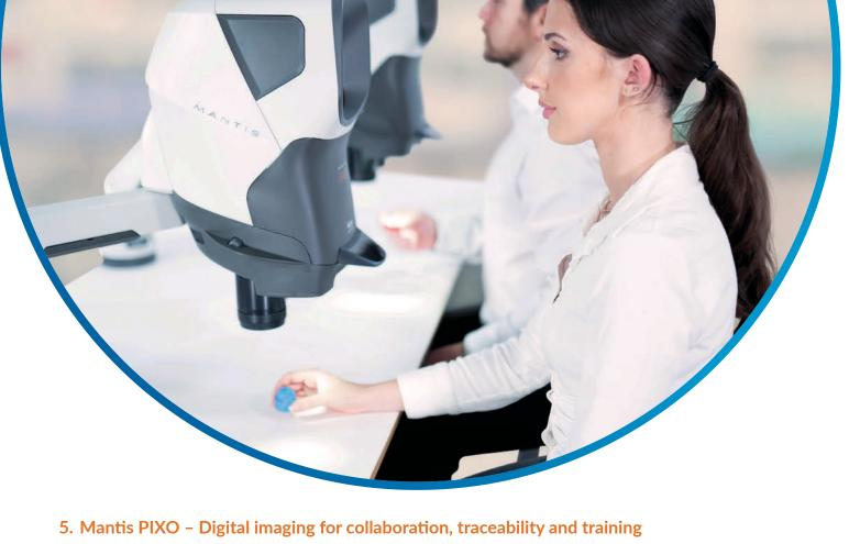
PIXO combines optical and digital technologies, providing perfect synergy between the optical stereo view and a high resolution camera. Capture, review and share detailed images for traceability, collaboration and training. Add text, shapes, arrows or digital overlays. Compare live images with targets, measures or pre-set guides.
